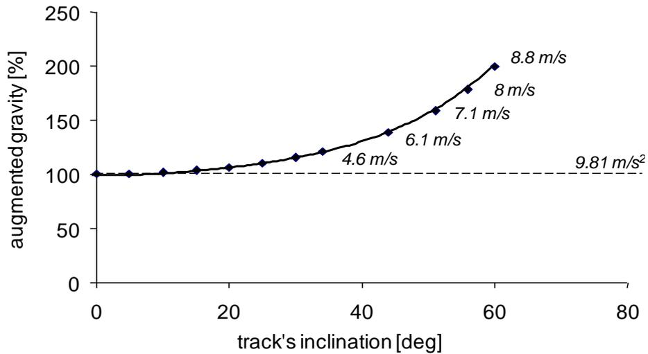
Figure 2. Graphical representation of the law governing the dynamics of running on the centrifugal track.
