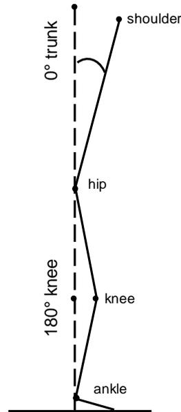
**Figure 6.** Angular convention used for expressing trunk and knee kinematics.
